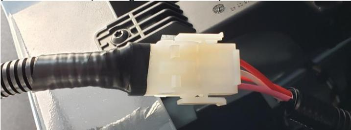
2. Unplug the 3-pin connector and insert the relay harness, as shown below:
